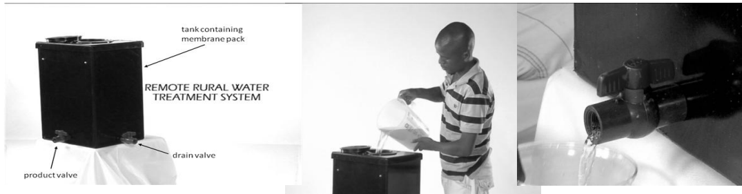
Figure 3: Rural Water Treatment Unit and Its Operation
